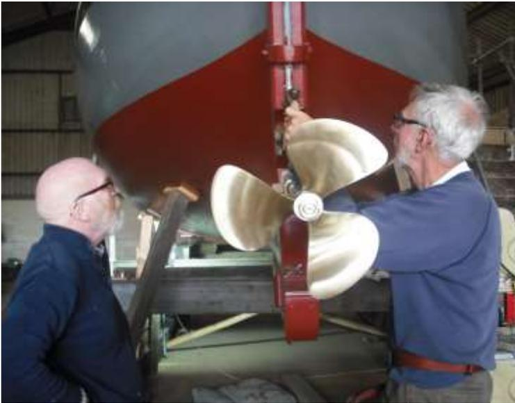
Tim Clayton (left) and Chris Ward offer up the shiny new propeller and propshaft on 29 June to find that the fit is good, and only minor adjustments were necessary before the rudder could be fitted. Tim's son Ed filmed the process – see it now on Youtube: [www.youtube.com/watch?v=ppjy\\_sFMRWw](http://www.youtube.com/watch?v=ppjy_sFMRWw) or on our website, above.
